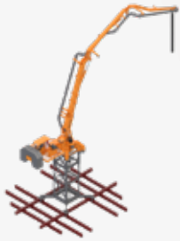
Tower Base Anchored to Deck (Anchored)
